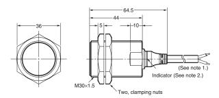
Note 1. 4-dia. vinyl-insulated round cable with 3 conductors (conductor cross section: 0.3 mm²; insulator diameter: 1.3 mm); standard length: 2 m
