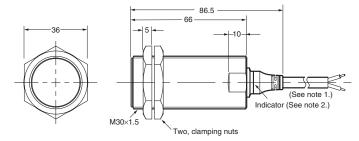
Note 1. 4-dia. vinyl-insulated round cable with 3 conductors (conductor cross section: 0.3 mm²; insulator diameter: 1.3 mm); standard length: 2 m
