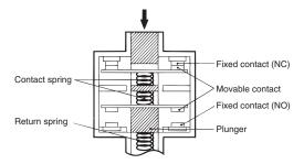
Conforms to EN60947-5-1 Direct Opening . (Only the NC contacts have a direct opening function.) When metal weld occurs, the NC contacts are separated from each other by pushing in the plunger.
