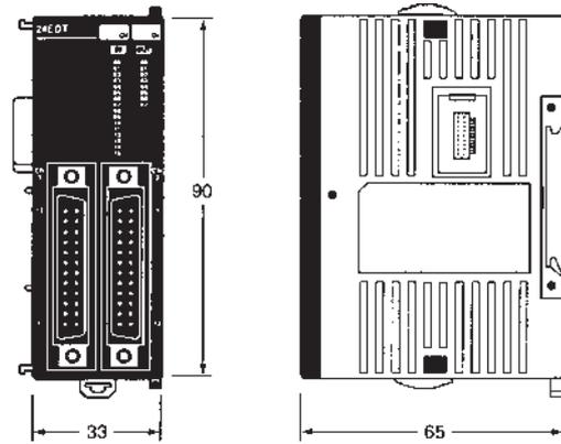
Units with Transistor Outputs Only and Units with Inputs Only
