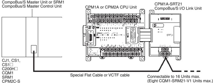
**Note:** A single CompoBus/S I/O Link Unit together with a maximum of two other Expansion I/O Units can be connected to the CPM1A or CPM2A CPU Unit.
