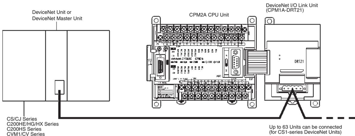
**Note:** Up to 3 DeviceNet I/O Link Units and other Expansion I/O Units can be mounted to CPM1A/CPM2A CPU Units.
