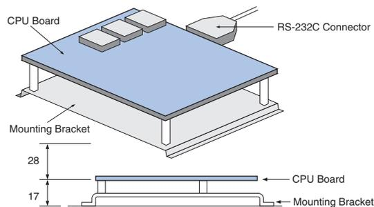
**Note:** Dimensions using a CPU Board. Horizontal expansion using CPM2B-CN411 Cable with an Expansion Board is possible.
