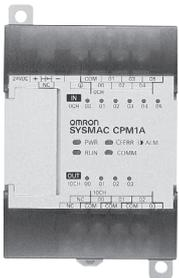
Setting a standard for micro PLCs, the CPM1A packs all basic functions into a compact size. Four CPU sizes are available, each with a choice of AC or DC power, relay or transistor outputs. Select any combination of power supply, output, and the number of I/O points to meet your needs.
