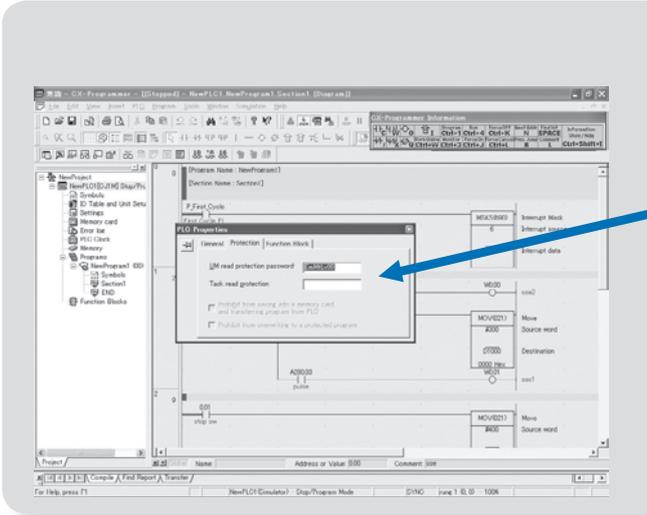
Programs can be protected by setting a password from the CX-Programmer (with the PLC online).
