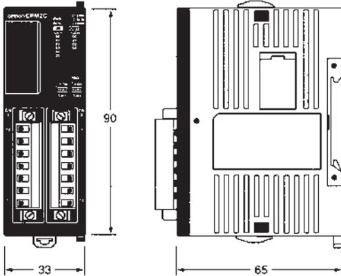
**CPU Units with Transistor Outputs**
