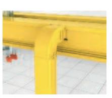
Mounting of vertical exit of system size 50 If the cable volume is even greater, then it is advisable to use trunking sections for vertical cable exits. These can be filled and then closed with the cover. This means there is no need to draw in the cables and that simple retroinstallation is possible.
