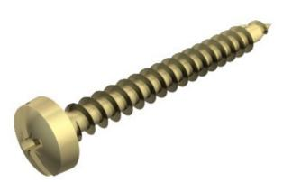
Hardened steel, electrogalvanised and yellow passivated, as well as Hostafloncoated, panhead with combined Philips and slotted head (Pozidrive size 2 except Ø 6 mm Pozidrive size 3).
