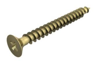
Hardened steel, electrogalvanised and yellow passivated, as well as Hostaflon-coated, countersunk head with Philips head (Pozidrive size 2 except  $\emptyset$  6 mm Pozidrive size 3).
