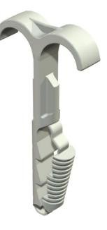
Save time and effor – with the highly flexible OBO plug-in anchor system. All you need is to drill hole with a diameter of 6 m. Then you can simply push the different push-fit anchors into the drill holes by hand – with the minimum of force.
