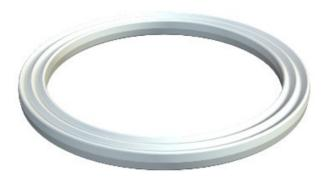
Connection thread sealing ring, in accordance with Part 9 to DIN 46320, however, dimensions may, according to material or function, deviate, suitable for all plastic cable glands with PG connection thread to DIN en 40430, the internal diameter of the sealing rings are designed so that they can be captively pre-mounted.
