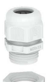
The quickest and most convenient way of providing strain relief and tightness with cable glands on junction boxes and housings is with the tried-and-trusted V-TEC VM cable glands from OBO. With the integrated sealing lip and the special OBO lamella technology protection class IP68 is achieved. Strain relief and tightness have been tested to DIN en 50262.
