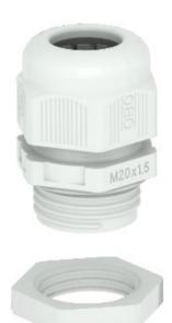
The quickest and most convenient way of providing strain relief and tightness with cable glands on junction boxes and housings is with the tried-and-trusted V-TEC VM cable glands from OBO. With the integrated sealing lip and the special OBO lamella technology protection class IP68 is achieved. Strain relief and tightness have been tested to DIN en 50262.
