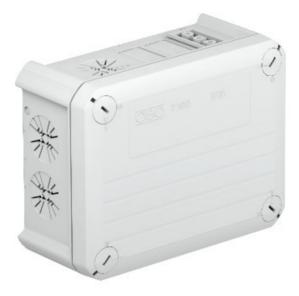
All the T series junction boxes are UV-resistant. They are made of polypropylene (thermoplastic polymer) and are equipped with strain relief entries and preterminated Wieland connection sockets, type GST-18-i3 (s = black, w = white, r = red). The strain relief entries can be penetrated directly with the cables. The special structure of the opening means that the cables cannot be removed unintentionally. Suitable for cable diameters of between 7 and 21 mm
