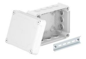
The junction boxes consist of thermoplastic material. The bottom parts are made from impact-resistant polypropylene, the box cover is made from extremely hard-wearing, impact-resistant polycarbonate. The high IK 10 impact resistance at -5°C shows this also.
