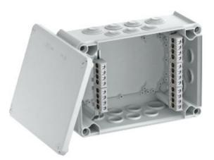
All the T series junction boxes are UV-resistant. They are made of a thermoplastic polypropylene plastic with plug-in seals made of ethylene vinyl acetate (EVA). This plastic is soft, which means that it is malleable. This allows installation of cables through the 16x M32 + 8x M40 seals, or the seals can be cut with a knife at the premarked points, in order to create an insertion opening for cables or pipes.
