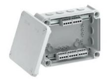
The junction boxes are made of a thermoplastic polypropylene polymer with plug-in seals made of ethylene vinyl acetate (EVA). This allows installation of cables either directly through the 7x M25 + 5x M32 seals, or the seals can be cut with a knife at the pre-marked points, in order to create an insertion opening for cables or pipes. Alternatively, cable glands can be pushed through the openings instead of the seals and locked with a locknut from the inside.
