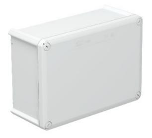
The junction boxes are made of a thermoplastic polypropylene polymer with closed side walls. This means that the required openings can be made wherever they are required. EDK plug-in seals or cable glands with locknuts can be inserted in these openings, to allow cable insertion.
