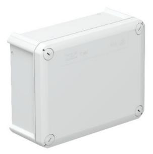
The junction boxes are made of a thermoplastic polypropylene polymer with closed side walls. This means that the required openings can be made wherever they are required. EDK plug-in seals or cable glands with locknuts can be inserted in these openings, to allow cable insertion.
