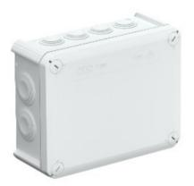
The junction boxes are made of a thermoplastic polypropylene polymer with plug-in seals made of ethylene vinyl acetate (EVA). This allows installation of cables either directly through the 7x M25 + 5x M32 seals, or the seals can be cut with a knife at the pre-marked points, in order to create an insertion opening for cables or pipes. Alternatively, cable glands can be pushed through the openings instead of the seals and locked with a locknut from the inside.
