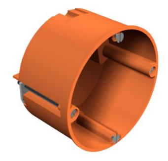
Cavity wall accessory socket. Dimensions to DIN 49073-1, for plate thickness 7-35 mm Standard combination spacing 71 mm, option for continuous wiring using connection support for combinations between accessory sockets and accessory connection sockets, 8 break-out openings for NYM cables, data cables and pipes Ø 20 mm, accessory sockets can also be used as connection sockets to VDE 0606-1 with double bolt fastening and screw-on cover, protection rating IP20.
