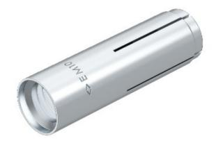
The drop-in anchor And can be used for single fixings in non-cracked concrete as well as for multiple fixings in cracked concrete of non-load-bearing systems. The setting tool is placed onto the anchor sleeve thereby creating a visible mark which confirms the correct installation. Through the controlled expansion, the necessary axial spacings and edge distances are decreased significantly.
