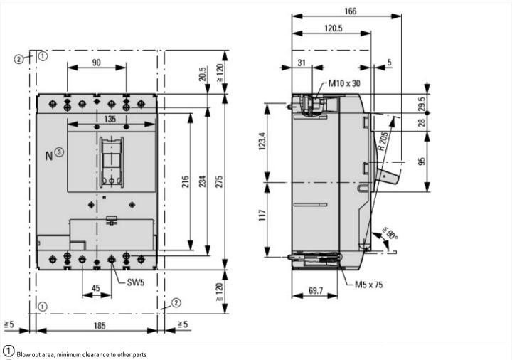
$\textcircled{2}_{\text{Minimum clearance to adjacent parts}}$
