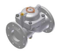
Cooling water regulating valves of type WVTS are suitable for controlling the temperature of a flow of water or neutral brine. WVTS water reg. valve opens on rising sensor temperature. Large self-acting cooling water regulating valves for accurate flow control based on sensor temperature Open on rising temperature Cast iron valve body Thermostatic pilot elements (2 or 5 m capillary tube) ordered separately
