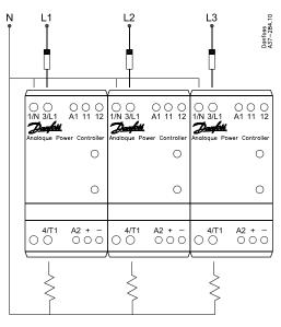
Max. load at: 230 V 3 x ACI 30-1 20.7 kW 3 x ACI 50-1 34.5 kW Three phase with single-phase contactor ECI-1 as slave Only burst firing mode
