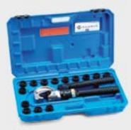
The built-in safety valve will by-pass the oil supply when the maximum pressure is reached, and a pressure release system can easily be operated at any stage of the compression.
