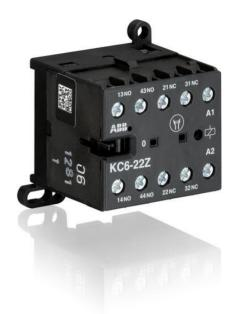
The KC6-22Z mini contactor relay is a compact 4 pole contactor relay with screw terminals. They are ideally suited for applications where reliability is a must and space is at a premium. Mini contactors relays are used in residential buldings, commercial buildings and industrial applications for switching of control signals up to 3 A / 400 V (AC-15). Further features are the noiseless and hum-free coil and a a switch position indication.
