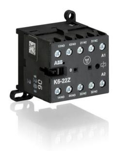
The K6-22Z mini contactor relay is a compact 4 pole contactor relay with screw terminals. They are ideally suited for applications where reliability is a must and space is at a premium. Mini contactors relays are used in residential buldings, commercial buildings and industrial applications for switching of control signals up to 3 A / 400 V (AC-15). Further features are the silent coil, a switch position indication and the integrated possibility for rail or wall mounting.
