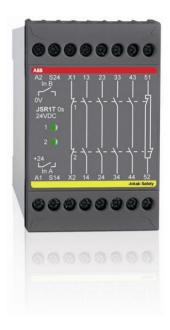
Safety expansion relay - for expanding the outputs of safety relays. Time delay 10 sec. Relay outputs 4NO/1NC
