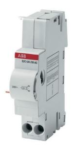
The S2C-UA 24 DC undervoltage release has the function to protect the load in case of a voltage drop included between 70% and 35% of its rated value. Positive safety (device tripping when the voltage is disconnected) emergency stop by means of a button. Suitable for MCBs S200 series, RCCBs F200 series and RCBOs DS201, DS202C, DS200 series. It can be used with MCBs SN201 series by means of SN201-IH interface module. Rated voltage: 24V d.c.
