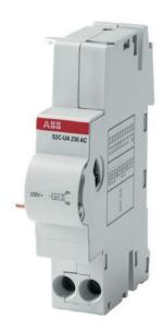
The S2C-UA 400 AC undervoltage release has the function to protect the load in case of a voltage drop included between 70% and 35% of its rated value. Positive safety (device tripping when the voltage is disconnected) emergency stop by means of a button. Suitable for MCBs S200 series, RCCBs F200 series and RCBOs DS201, DS202C, DS200 series. It can be used with MCBs SN201 series by means of SN201-IH interface module. Rated voltage: 400V a.c.
