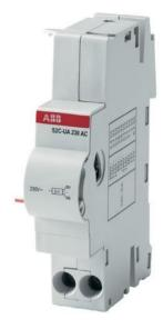
The S2C-UA 12 DC undervoltage release has the function to protect the load in case of a voltage drop included between 70% and 35% of its rated value. Positive safety (device tripping when the voltage is disconnected) emergency stop by means of a button. Suitable for MCBs S200 series, RCCBs F200 series and RCBOs DS201, DS202C, DS200 series. It can be used with MCBs SN201 series by means of SN201-IH interface module. Rated voltage: 12V d.c.
