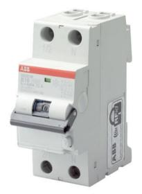
The DS201 series RCBO is a 1P+N in two-modules device for the protection of end user single-phase circuits against overload and short-circuit currents; provides an optimal trade-off between safety and continuity of service, thanks to the resistance to unwanted trippings; protection against indirect contacts and additional protection against direct contacts (with sensitivity = 30 mA); protection and isolation of resistive and inductive loads.
