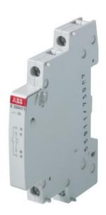
E250 allows contact switching for each impulse sent to coil, using normally open pushbuttons. Ideal for lamp remote controlling from different positions. They also allow manual operations on the product.
