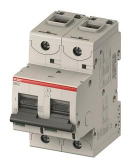
The S802PV-M63-H is a 2-pole polarized disconnector for photovoltaics. It can be used for currents up to 63A and has a rated operational voltage of 1000V DC by only 54mm width. The rated short-term withstand current Icw is 1.5kA. The S802PV-M63-H complies with IEC/EN 60947-3. It has numerous of approvals, therefore it can be used worldwide. The extensive range of accessory makes the use of S802PV-M63-H more comfortable.
