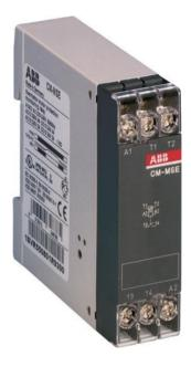
The CM-MSE relay is from the CM thermistor motor protection relay range. This relay operates with a rated control supply voltage of 220-240 V AC and has a 1 n/o output contact rated at 250 V / 4 A. It features one sensor circuit for monitoring of PTC temperature sensors or bimetals. This relay offers automatic reset and works according to the closed-circuit principle. A sealable transparent cover for protection against unauthorized changes is available as accessory
