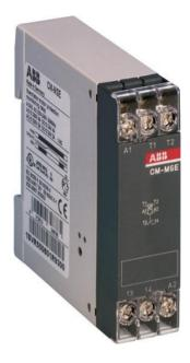
The CM-MSE relay is from the CM thermistor motor protection relay range. This relay operates with a rated control supply voltage of 110-130 V AC and has a 1 n/o output contact rated at 250 V / 4 A. It features one sensor circuit for monitoring of PTC temperature sensors or bimetals. This relay offers automatic reset and works according to the closed-circuit principle. A sealable transparent cover for protection against unauthorized changes is available as accessory
