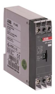
The CT-AKE is a single-function electronic time relay from the CT-E timer range. It provides an OFF-delay (delay on break) function with a time range from 0.3 s to 30 s. This time relay operates with a rated control supply voltage of 24 - 240 V AC / DC and has a solid-state output.
