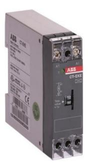
The CT-EKE is a single-function electronic time relay from the CT-E timer range. It provides an ON-delay (delay on make) function with a time range from  $0.1 \, \text{s}$  to  $10 \, \text{s}$ . This time relay operates with a rated control supply voltage of  $24 - 240 \, \text{V}$  AC / DC and has a solid-state output.
