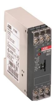
The CT-SDE is a single-function electronic time relay from the CT-E timer range. It provides a star-delta function with a time range from 0.3 s to 30 s. This time relay operates with a rated control supply voltage of 110 - 130 V AC and has a 1 n/o + 1 n/c output with contacts rated at 250 V / 4 A.
