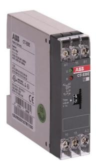
The CT-EBE is a single-function electronic time relay from the CT-E timer range. It provides a flasher (recycling equal times) function with a time range from  $0.1 \, \text{s}$  to  $10 \, \text{s}$ . This time relay operates with a rated control supply voltage of  $220 - 240 \, \text{V}$  AC and has a  $1 \, \text{c/o}$  (SPDT) output rated at  $250 \, \text{V}$  /  $4 \, \text{A}$ .
