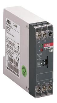
The CT-AWE is a single-function electronic time relay from the CT-E timer range. It provides an impulse-OFF (trailing edge interval) function with a time range from 0.05 s to 1 s. This time relay operates with a rated control supply voltage of 110 - 130 V AC and has a 1 c/o (SPDT) output rated at 250 V / 4 A. A control input works with voltage-related (non-floating) triggering.
