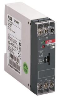
The CT-AWE is a single-function electronic time relay from the CT-E timer range. It provides an impulse-OFF (trailing edge interval) function with a time range from 3 s to 300 s. This time relay operates with a rated control supply voltage of 24 V AC / DC and has a 1 c/o (SPDT) output rated at 250 V / 4 A. A control input works with voltage-related (non-floating) triggering.
