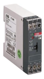
The CT-AWE is a single-function electronic time relay from the CT-E timer range. It provides an impulse-OFF (trailing edge interval) function with a time range from 0.3 s to 30 s. This time relay operates with a rated control supply voltage of 220 - 240 V AC and has a 1 c/o (SPDT) output rated at 250 V / 4 A. A control input works with voltage-related (non-floating) triggering.
