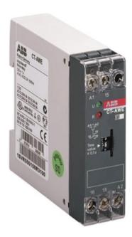
The CT-AWE is a single-function electronic time relay from the CT-E timer range. It provides an impulse-OFF (trailing edge interval) function with a time range from 3 s to 300 s. This time relay operates with a rated control supply voltage of 110 - 130 V AC and has a 1 c/o (SPDT) output rated at 250 V / 4 A. A control input works with voltage-related (non-floating) triggering.
