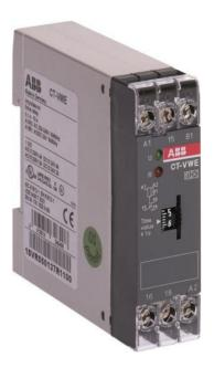
The CT-VWE is a single-function electronic time relay from the CT-E timer range. It provides an impulse-ON (interval) function with a time range from 3 s to 300 s. This time relay operates with a rated control supply voltage of 110 - 130 V AC and has a 1 c/o (SPDT) output rated at 250 V / 4 A.
