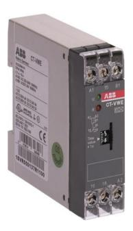
The CT-VWE is a single-function electronic time relay from the CT-E timer range. It provides an impulse-ON (interval) function with a time range from  $0.1 \, s$  to  $10 \, s$ . This time relay operates with a rated control supply voltage of  $110 - 130 \, V$  AC and has a 1 c/o (SPDT) output rated at  $250 \, V$  /  $4 \, A$ .
