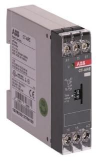
The CT-ARE is a single-function electronic time relay from the CT-E timer range. It provides an OFF-delay (true delay on break) function without auxiliary voltage and with a time range from 0.3 s to 30 s. This time relay operates with a rated control supply voltage of 24 V AC / DC / 220 - 240 V AC and has a 1 c/o (SPDT) output rated at 250 V / 4 A.
