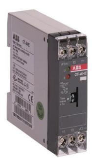
The CT-AHE is a single-function electronic time relay from the CT-E timer range. It provides an OFF-delay (delay on break) function with a time range from 0.3 s to 30 s. This time relay operates with a rated control supply voltage of 24 V AC / DC and has a 1 c/o (SPDT) output rated at 250 V / 4 A. A control input works with voltage-related (non-floating) triggering.
