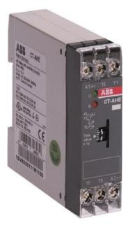
The CT-AHE is a single-function electronic time relay from the CT-E timer range. It provides an OFF-delay (delay on break) function with a time range from 0.3 s to 30 s. This time relay operates with a rated control supply voltage of 220 - 240 V AC and has a 1 c/o (SPDT) output rated at 250 V / 4 A. A control input works with voltage-related (non-floating) triggering.
