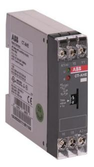
The CT-AHE is a single-function electronic time relay from the CT-E timer range. It provides an OFF-delay (delay on break) function with a time range from 0.1~s to 10~s. This time relay operates with a rated control supply voltage of 220~-240~V AC and has a 1~c/o (SPDT) output rated at 250~V / 4~A. A control input works with voltage-related (non-floating) triggering.
