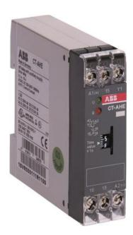
The CT-AHE is a single-function electronic time relay from the CT-E timer range. It provides an OFF-delay (delay on break) function with a time range from 3 s to 300 s. This time relay operates with a rated control supply voltage of 110 - 130 V AC and has a 1 c/o (SPDT) output rated at 250 V / 4 A. A control input works with voltage-related (non-floating) triggering.
