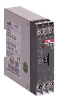
The CT-ERE is a single-function electronic time relay from the CT-E timer range. It provides an ON-delay (delay on make) function with a time range from 3 s to 300 s. This time relay operates with a rated control supply voltage of 24 V AC / DC / 220 - 240 V AC and has a 1 c/o (SPDT) output rated at 250 V / 4 A.
